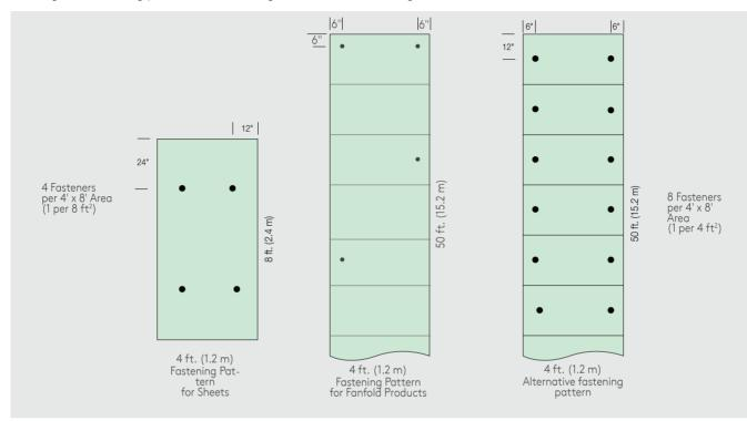
Fastening Patterns for Kingspan GreenGuard® Roofing Cover Board Used Under Dark-Colored Roof Membranes
