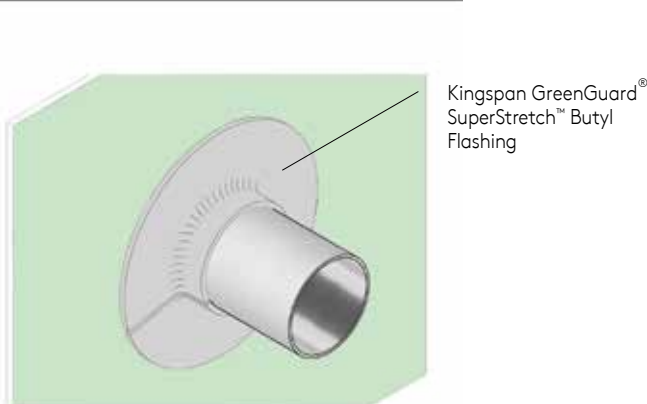
Figure 34: Installation of Flashing at Pipe Penetration
