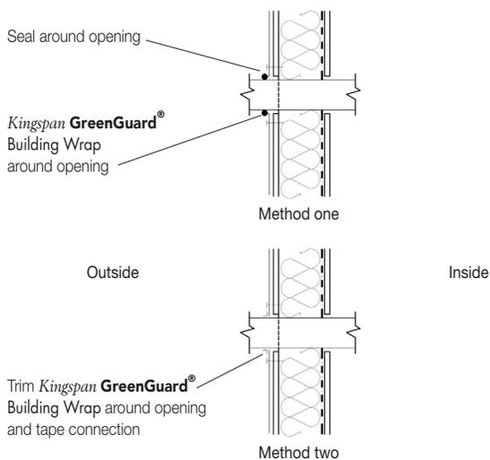
Figure 5: Installation of Building Wrap at Wall Penetrations
