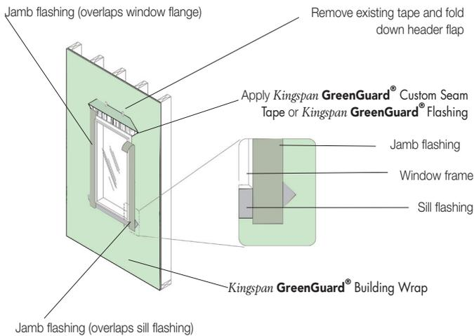
Figure 13: Tape Header Flap Down
