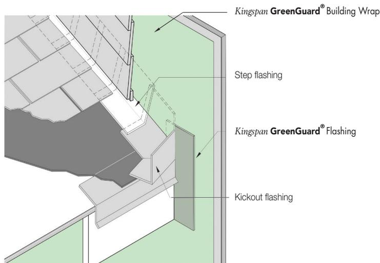
Figure 29: Kickout Flashing
