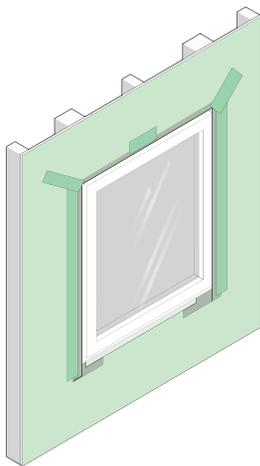
Figure 16: Sealing Building Wrap around Window
