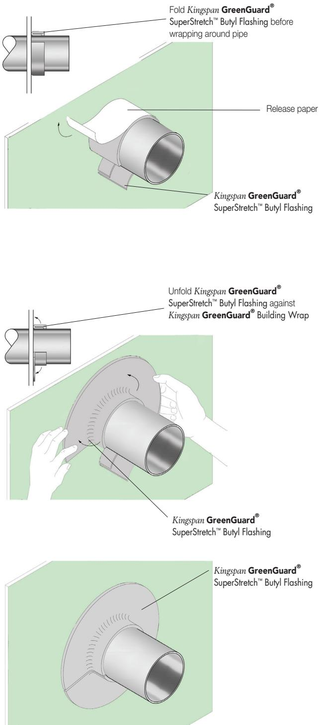
Figure 34: Installation of Flashing at Pipe Penetration
