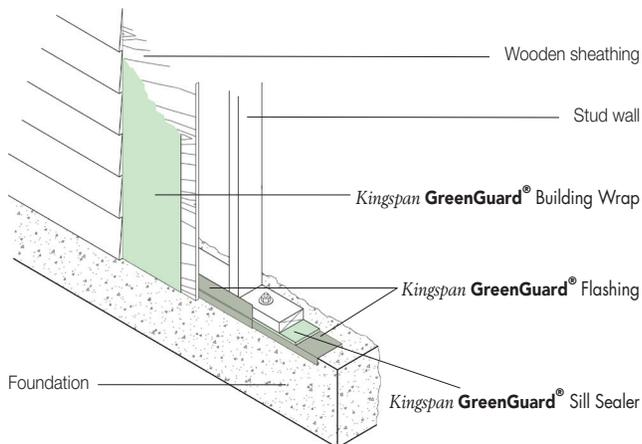
Figure 32: Installation of Flashing at Sill Plate
