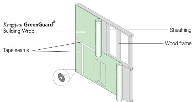
Figure 2: Exterior Wall with *Kingspan GreenGuard*® Building Wrap
