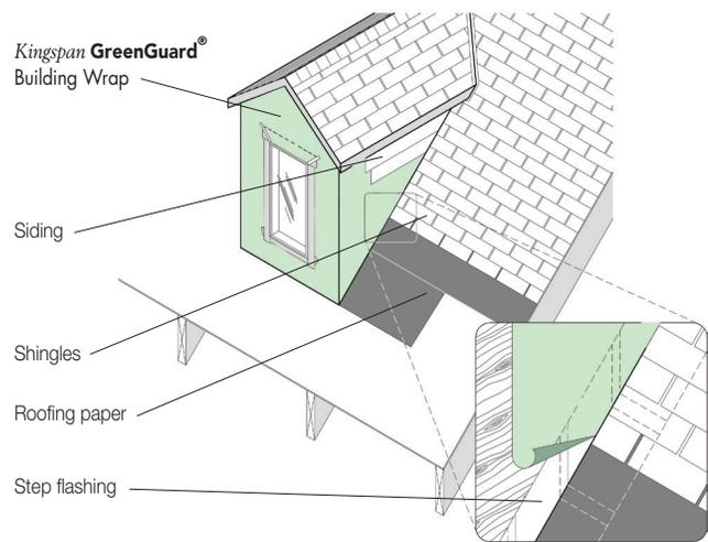
Figure 30: Installation of Building Wrap / Wall Intersection
