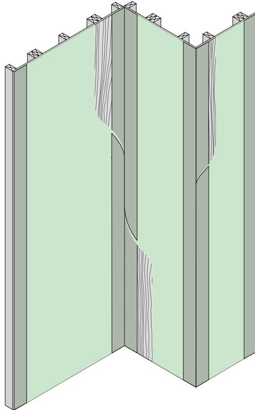
Figure 35: Flashing of Inside and Outside Corners
