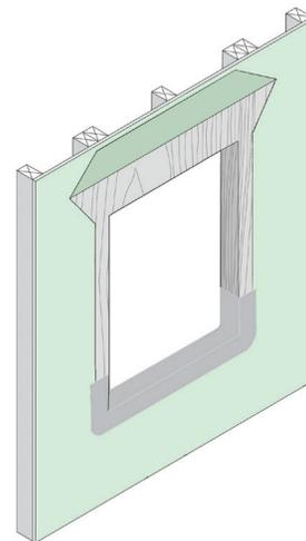
Figure 11: Cut Back of Wrap on the Sides
