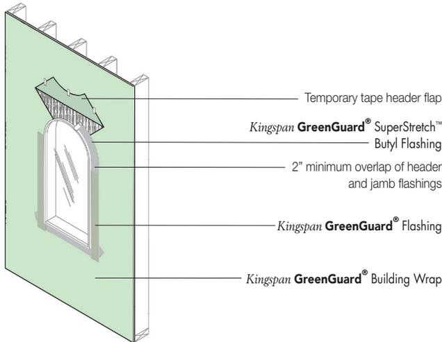
Figure 28: Installation of Flashing Arched Window
