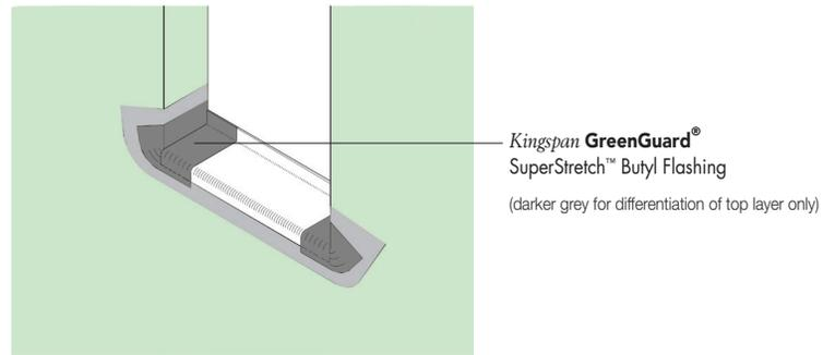
Figure 22: Sill Pan Option Corners Sealed
