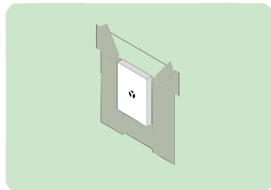
Figure 33: Installation of Flashing at Mounting Block
