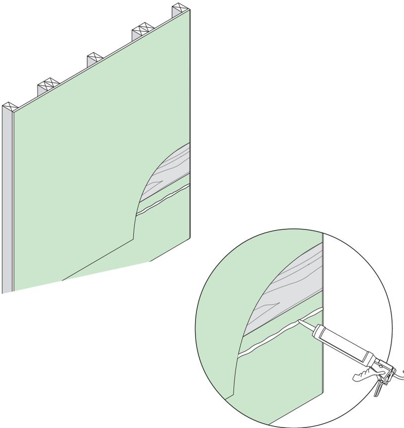
Figure 36: Using adhesive to seal building wrap.
