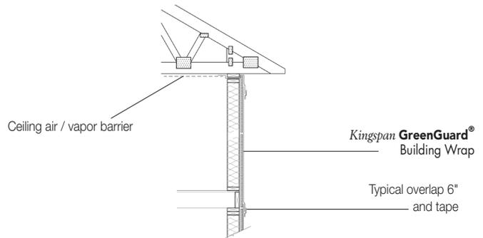
Figure 1: Exterior Wall Cross-Section
